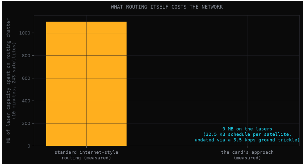
Figure 3.2.4. Modeled inter-satellite routing-control traffic over ten minutes. The zero bar excludes ground uploads and does not mean zero total networking overhead. Storage, upload rate and network-wide traffic are distinct metrics. Source: [2].
