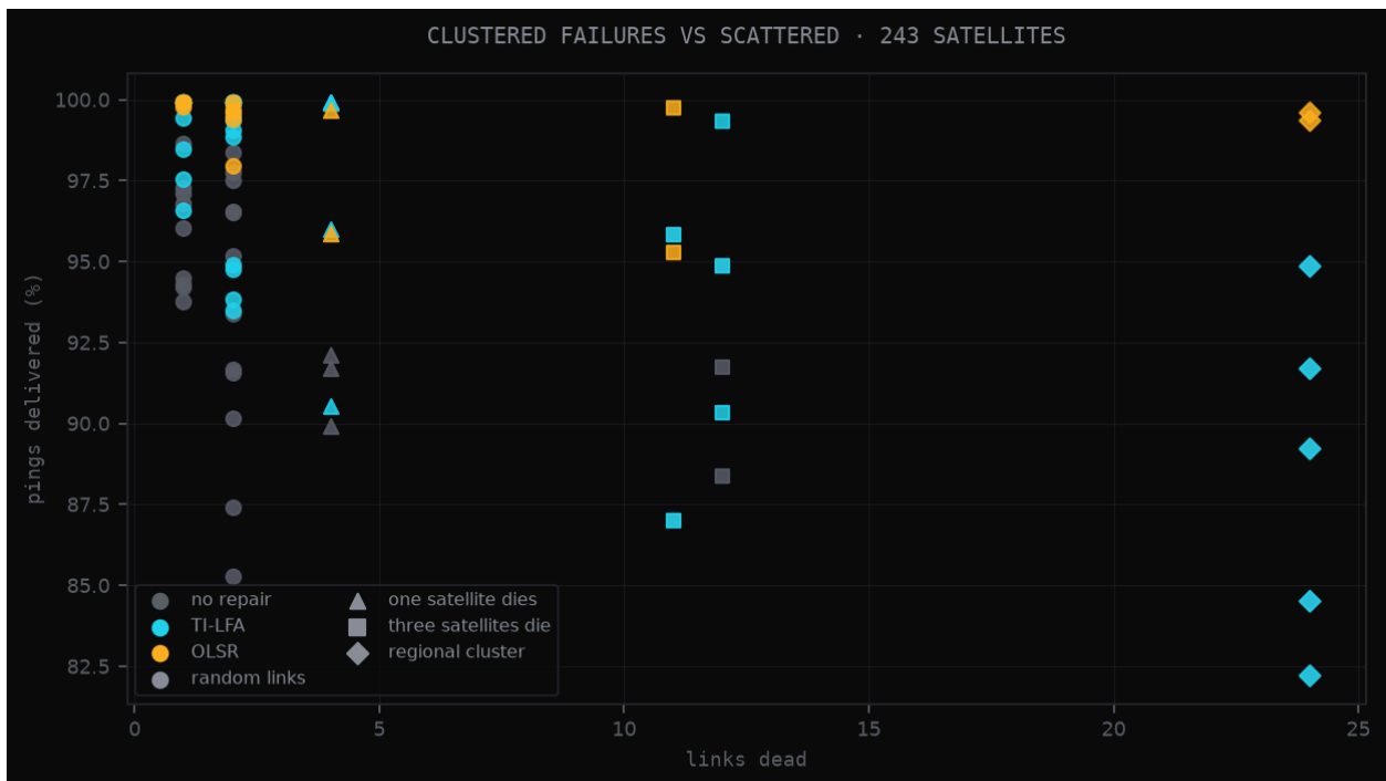
Figure 3.2.7. Delivery for random link losses, failed satellites and a regional cluster in the 243-satellite model. Comparisons apply to the particular failure locations and scenarios tested. Source: [2].
